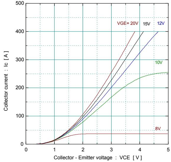
Collector current vs. Collector-Emiiter voltage
