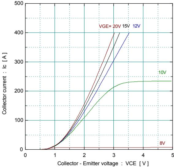
Collector current vs. Collector-Emiiter voltage
