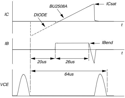
Fig.3. Switching times waveforms.
