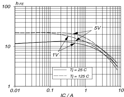
Fig.6. Typical DC current gain.  $h_{FE} = f (I_C)$  parameter  $V_{CE}$
