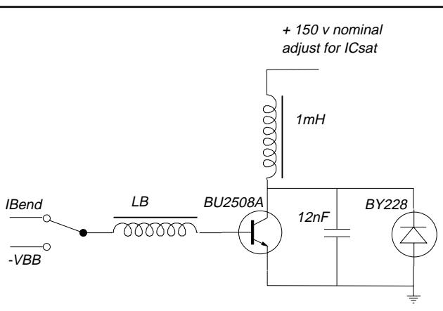
Fig.5. Switching times test circuit (BU2508A).
