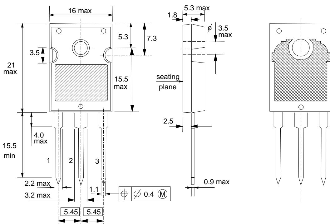
Fig.16. SOT429; pin 2 connected to mounting base.
