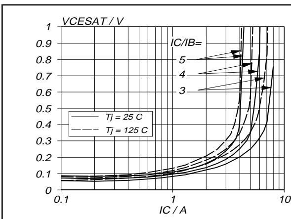
Fig.8. Typical collector-emitter saturation voltage.  $V_{CE\text{sat}} = f (I_C)$ ; parameter  $I_C/I_B$
