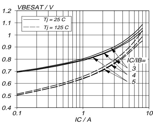
Fig.7. Typical base-emitter saturation voltage.  $V_{BE\text{sat}} = f (I_C)$ ; parameter  $I_C/I_B$
